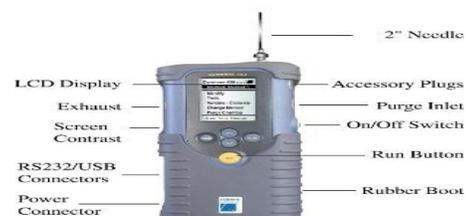
Fig.(8): Prototype of E-Nose (Cyrano).
