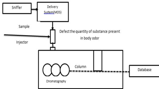
Fig.9: Block Diagram of Reception.
