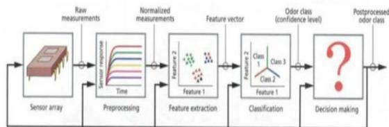
Fig. 11: Signal Processing and Pattern Recognition systems stages[4].
